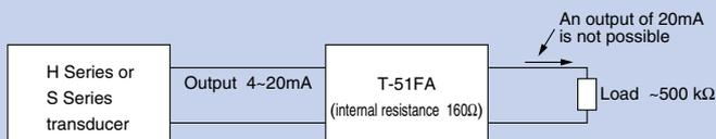
In the case shown to the left, the total load resistance connected to the output is 660Ω (500Ω+160Ω) and exceeds the allowable limit. For an output of 4~20mA, a load in the range of 0 to 440Ω can be connected to an H Series or S Series transducer.
