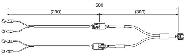
Split-type current sensor cable (3P4W)
