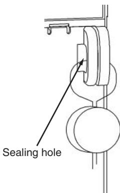
5 At sealing, seal the ETR cover by using the sealing hole at the top of the ETR cover.
