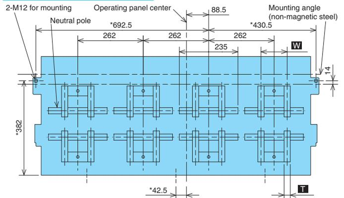
Fixed type AE630-SW, AE1000-SW, AE1250-SW, AE1600-SW
