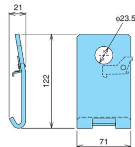
Fixed type AE2000-SW, AE2500-SW, AE3200-SW
