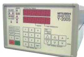
The electronic trip relay can be checked by this field test device when the breaker is at test position or disconnect position. The breaker will trip when tested with this device.
