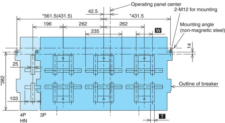
The mounting angle should be prepared by the customer.
