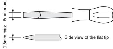
2 Insert the flat tipped screwdriver into the opening of the ETR cover. Then, lightly turn the screwdriver to the upside as shown in the left figure, and the ETR cover will open.
