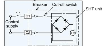
Diode rectifier is not used for control source 24-48V DC.
