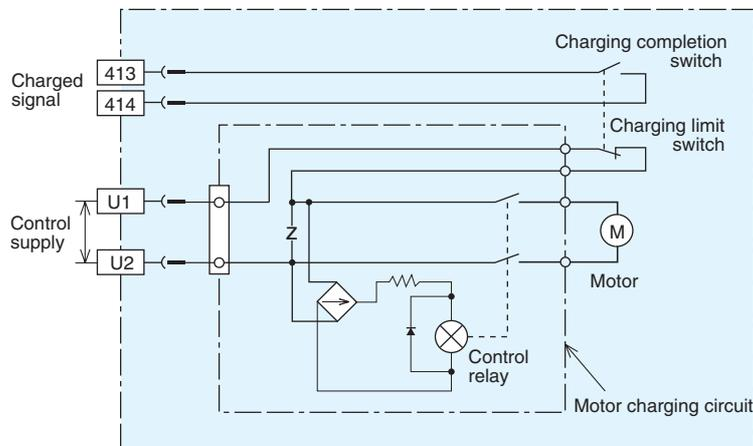
For 24V DC and 48V DC, the Diode rectifier is not included.
