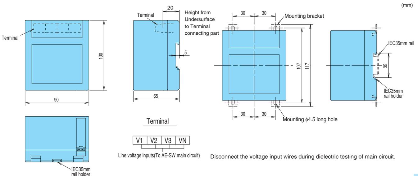
Disconnect the voltage input wires during dielectric testing of main circuit.
