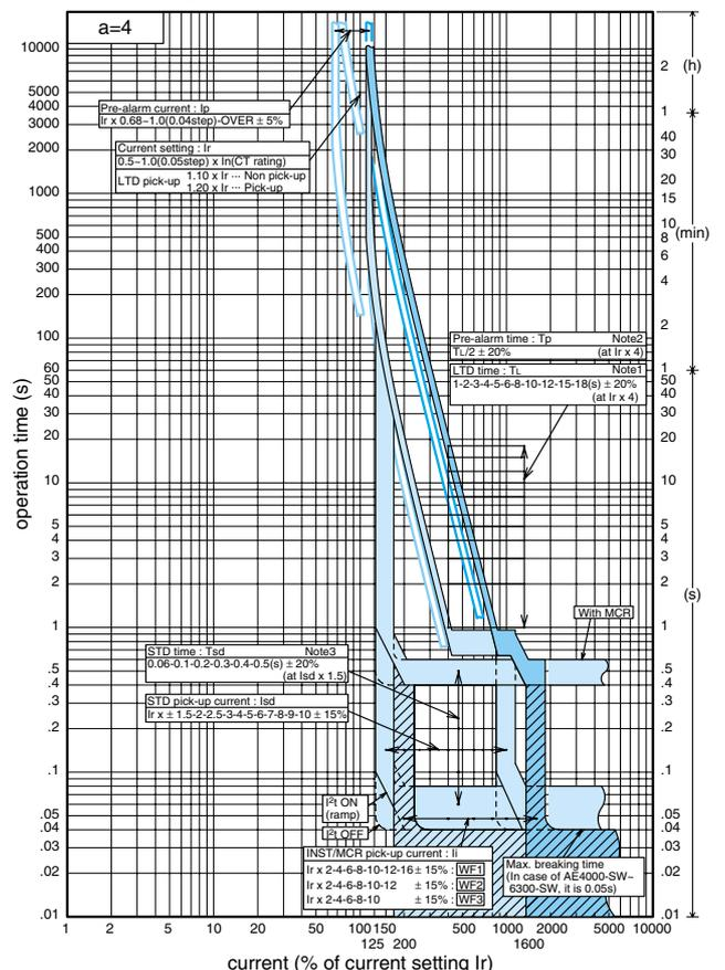
Note 1: LTD operating time  $t_{LTD}$  is calculated by the following equations.
